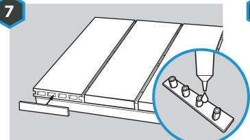
If using end caps, apply a high quality grab adhesive to the end caps to secure for extra adhesion. Wipe away any excess from the edge of the cap.
